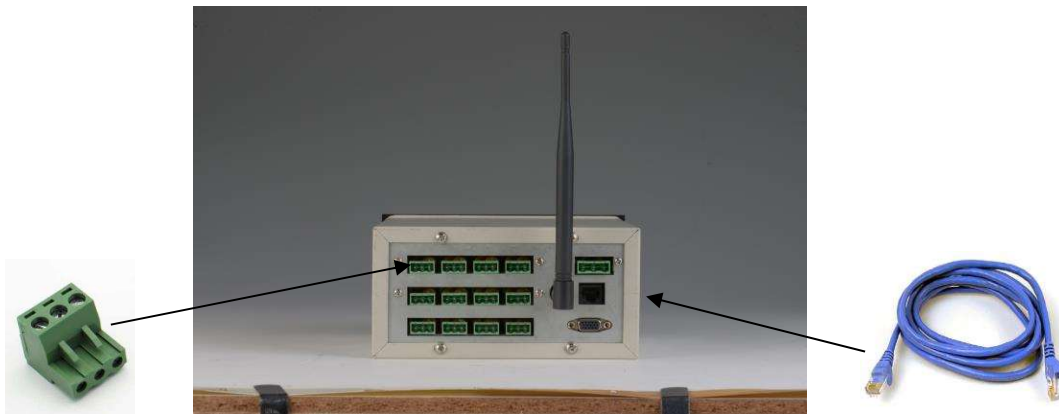
Figure 4 Relay and Ethernet Connection
